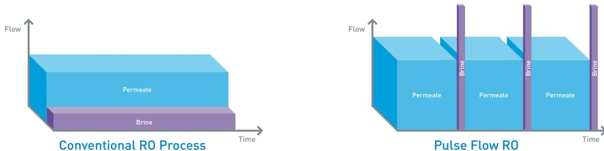
The diagram above presents the permeate and brine flow regime in conventional RO (left) and PFRO (right). PFRO operates in two cycles: production and flush. The pressure vessels continuously receive feed flow from the high-pressure pump and continuously produce permeate.
