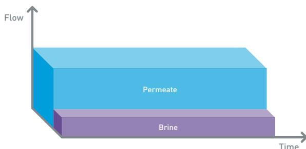
Brine flow is the minimum permitted by the membrane manufacturer. The flow is continuous and uninterrupted.
