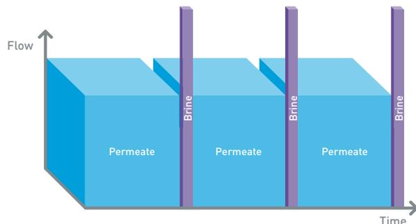
Brine flow discharges as pulses in a very short time at the maximum flow allowed by the membrane manufacturer.
